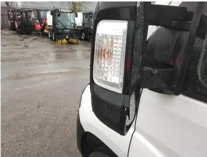
5: Door Mirror Assy nsf Broken Replace
