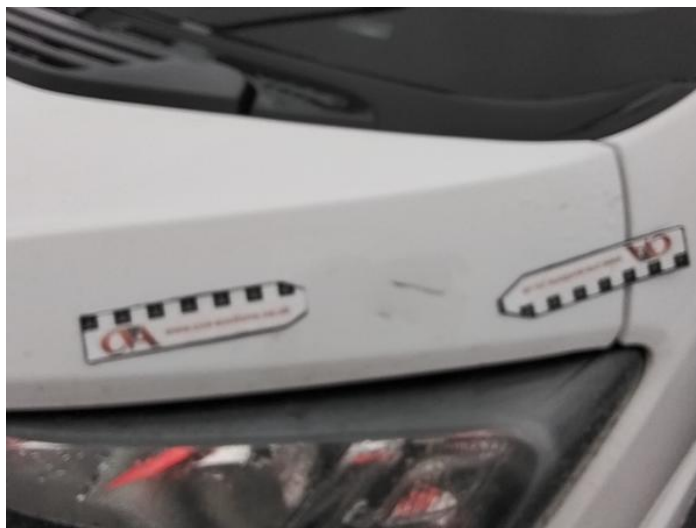
2: Bonnet Dented With Paint Damage
