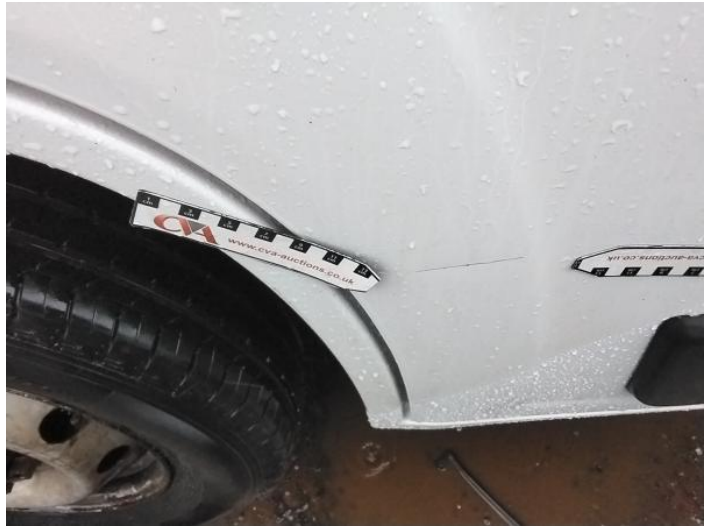
4: Door nsf Dented With Paint Damage
