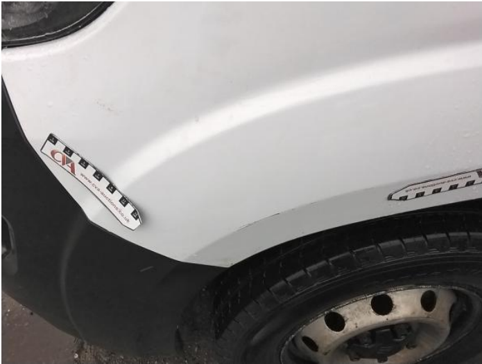
3: Wing nsf Scratched Over 25mm Thru Paint
