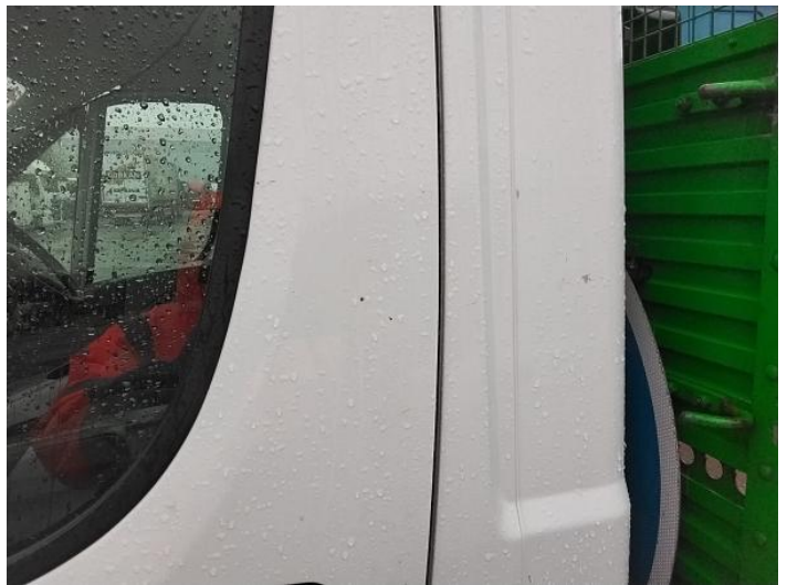
6: Door nsf Chipped Multiple Chips
