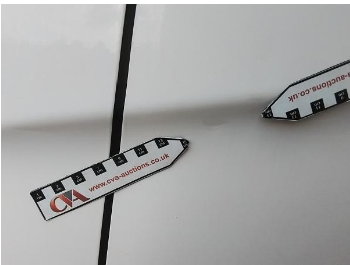
7: Door nsf Dented Over 30mm
