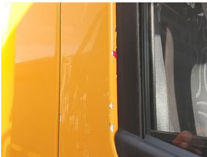
5: Door osf Chipped Multiple Chips
