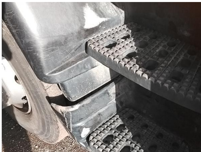
2: Moulding of Wing Scuffed (Unpainted) Over 100mm
